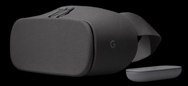
**Google Daydream View (2017)** relies on the phone for processing and tracking 3-DoF rotational only tracking of phone + controller
