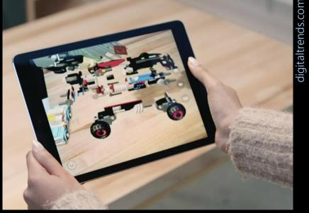
Apple ARKit (2017), Google ARCore (2018) visual-inertial odometry – combine inertial motion sensing with feature point tracking
