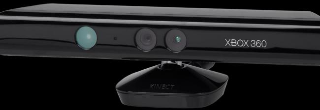
Microsoft Kinect (2010) IR laser speckle projector, RGB + IR cameras range: 1–6 m, accuracy: <5 mm 30 Hz update rate, 100 ms latency
