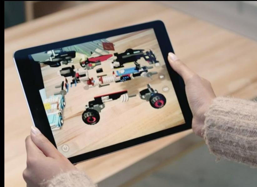
Apple ARKit (2017), Google ARCore (2018) visual-inertial odometry – combine inertial motion sensing with feature point tracking
