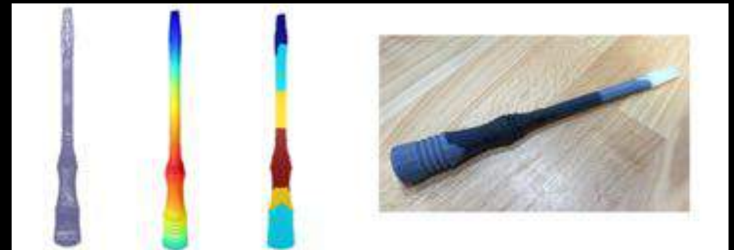
Screwdriver, 6 discrete parts and materials
